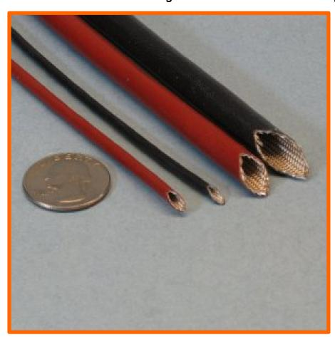
FlameShield™ small diameter firesleeve is designed as a primary insulation sleeve for protecting small diameter wire, cable, lines, hose, and pipe from high temperature, flame and environmental contamination. Recognized by UL / CSA for 240°C, 600V service, and complies with VW-1 flammability requirements. Conforms to, and is listed on the QPL for MIL-I-3190/9 (Grade A).
