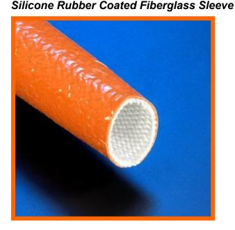
FlameShield™ Marine grade firesleeve allows properly assembled hose assemblies to meet ISO 15540 testing. We also maintain traceability records for customers buying this product. 500°F / 260°C continuous rating and with a 30 minute "Fireproof" 800°F / 426°C rating.
